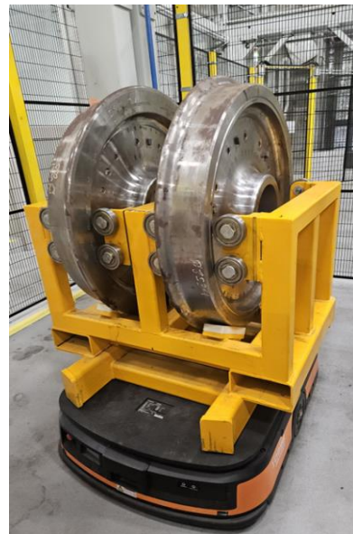
Fig. 6 - AGV for Wheel Blank Handling
