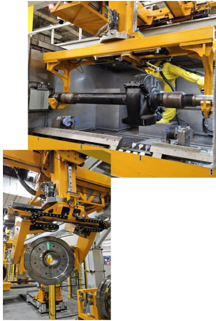
Fig. 5 - Wheelset and Wheel Blank Manipulators
