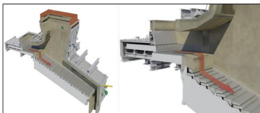
Fig. 4 - Typical Feeding-Grate Arrangement
