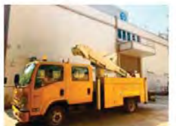
Insulated Elevating Work Platform (EWP)
