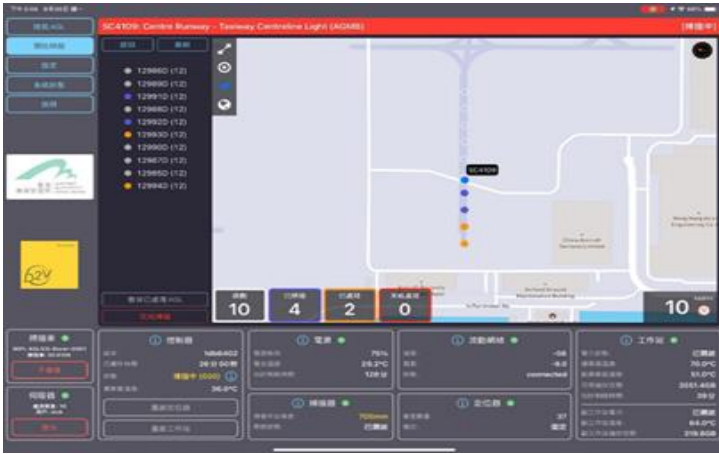
Fig. 17 - The Operator's Mobile Device enables the user to understand the Network and the Equipment Healthiness, pinpoint AGL locations for Inspection, Review Scanned AGLs, and assess Current and Past Inspection Outcomes, as shown in Fig. 1 to 5
