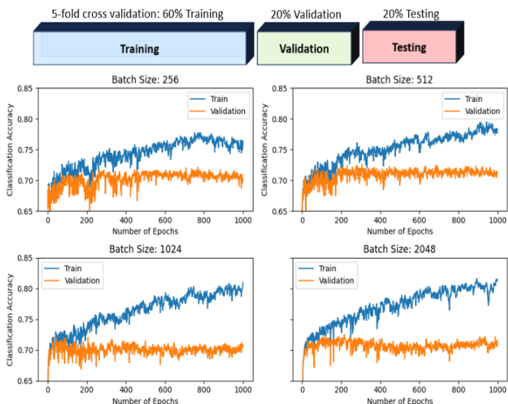
Fig. 3 - Validation Protocol and Learning Curves for Various Batch Sizes. Stratified 5-fold Cross Validation (CV) is Used
