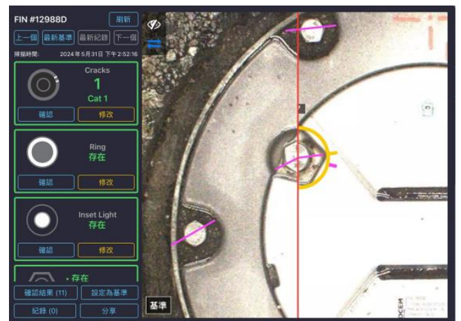
Fig. 2 - The Bolt Tightness was examined by Comparing the Inspection Photo with Historical Benchmark
