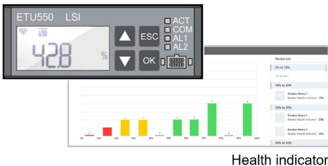
Fig. 15 - Health Indicator of Siemens Molded Case Circuit Breaker
