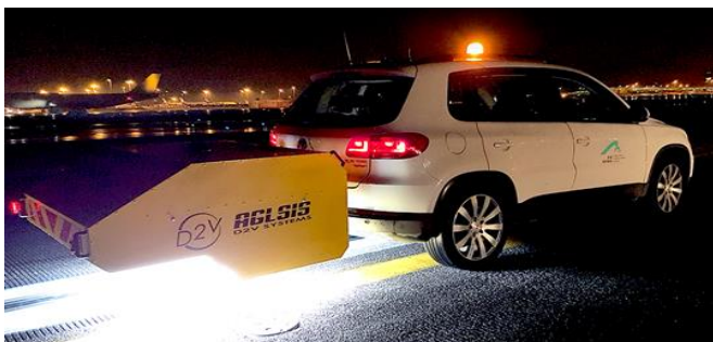
Fig. 6 - Proof-of-Concept Model: Inspection System developed as a Detachable Tool, required to install on a specific Inspection Vehicle
