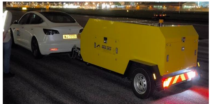
Fig. 7 - Inspection System converted to Trailer-based Universe Equipment, adaptable to various Towing Vehicles
