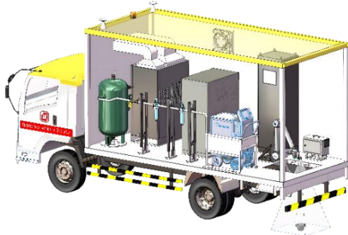
Fig. 11 - Conceptual Design of the Autonomous Airfield Ground Lighting Cleaning and Inspection Robot
