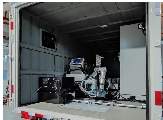
Fig. 13 - Prism Cleaning System of Autonomous Airfield Ground Lighting Cleaning and Inspection Robot
