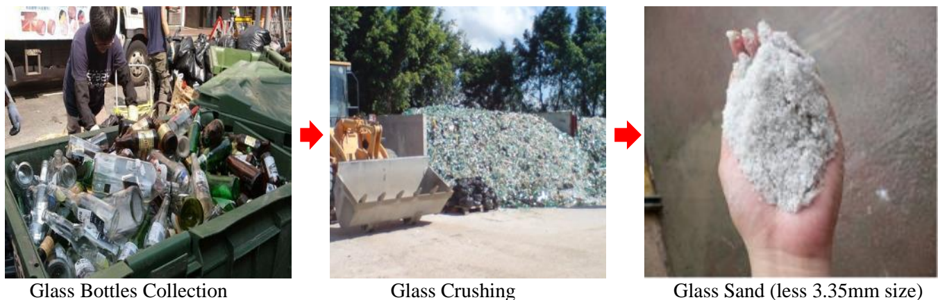
Figure 5: Glass Bottle Collection and Crushing Process
