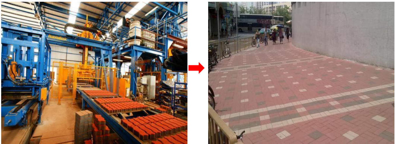
Figure 7: Eco-Glass Paving Block Manufacturing and Usage
