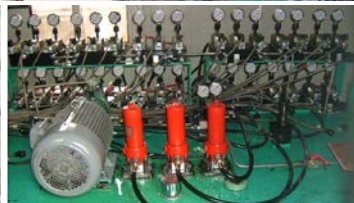
Innovation: Automatic Strut Load Compensation and Displacement Control System
