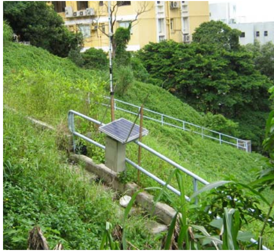
Figure 5: Base Station located at foot of slope
