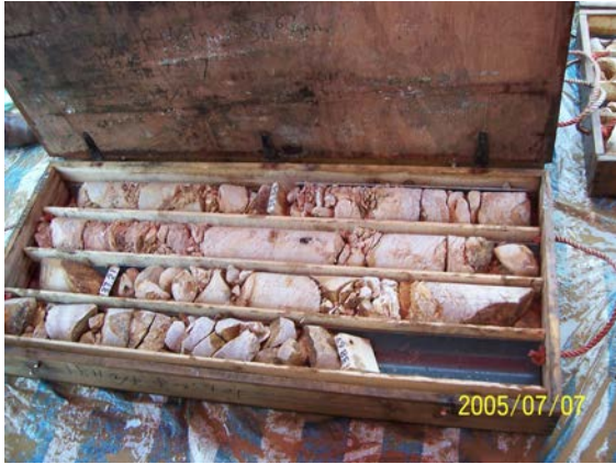
Figure 3: Rock quality at rock socket location of test pile
