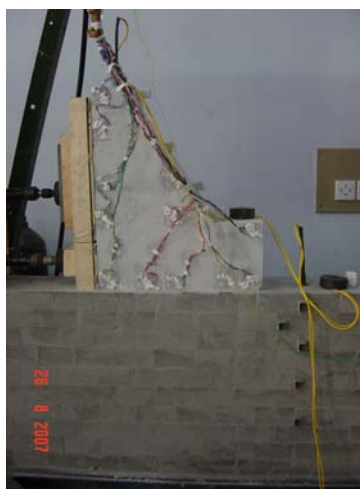
Figure 5: Installation of two FBG sensing bars for measuring displacement profiles
