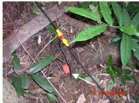
Geophone installed on ground & connected to a cable
