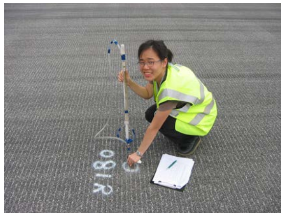
Figure 6: Manometer measured air pressure beneath asphalt
