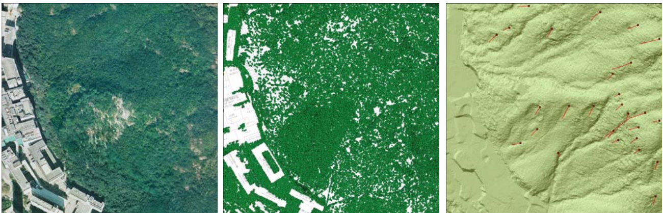
(a) Hillside in December 2006 (b) Ground points from LiDAR Survey (c) DEM generated using LiDAR data Figure 7: Generation of DEM of the natural hillside behind Queen Mary Hospital
