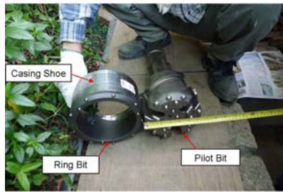
Plate 2: Ring bit and pilot bit for concentric drilling
