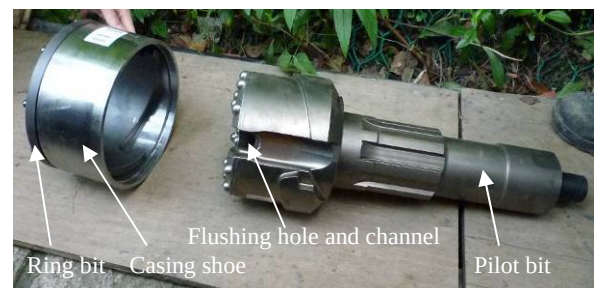
Plate 7: Ring bit and pilot bit of the concentric drilling system
