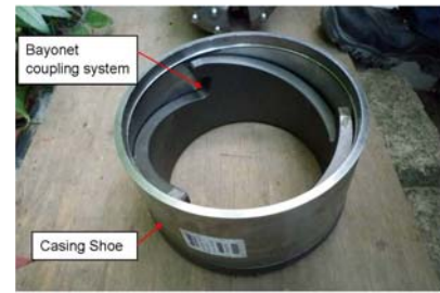
Plate 4: Spiral locking system for coupling the pilot bit and ring bit
