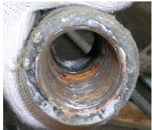
Plate 15: Rust formed in coupler
