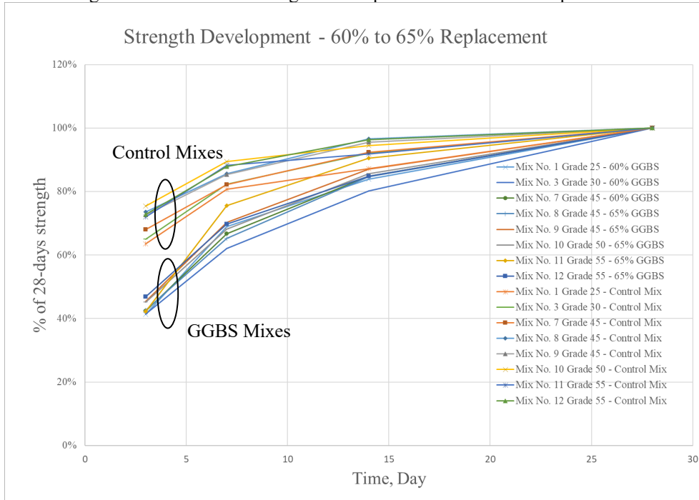
Figure 6 – GGBS Mix Strength Development – 60% to 65% Replacement
