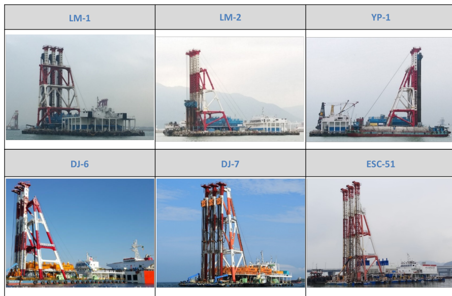
Figure 6: Marine DCM barges used in TCE project
