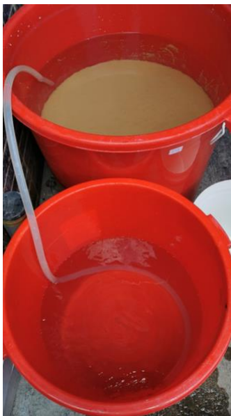
Plate 5: Step IV for recycling water from clay slurry and obtain clay material
