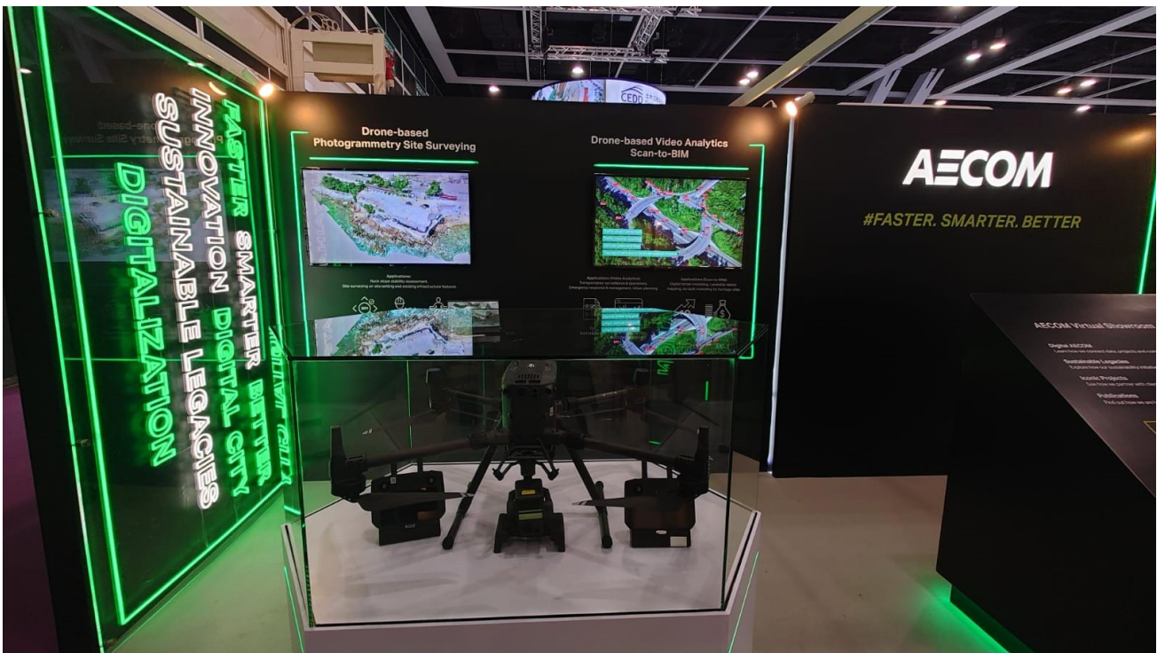
Plate 1: Unmanned Aerial Vehicle (UAV) equipped with Light Detection and Ranging (LiDAR) systems for digital terrain modelling and landslide mapping applications
