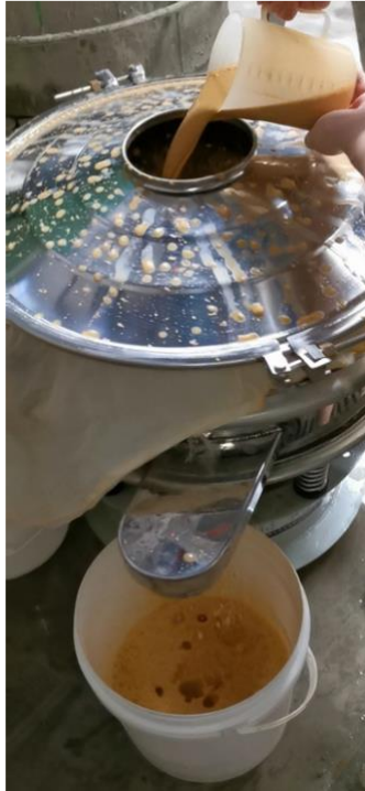
Plate 4: Step III for washing and sieving mud slurry into silt and clay slurry with water
