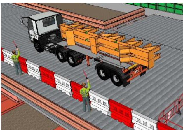
Figure 17 Digital Delivery of Modules to Site
