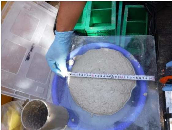
(a) Flowability test in accordance with ASTM D6103-17
