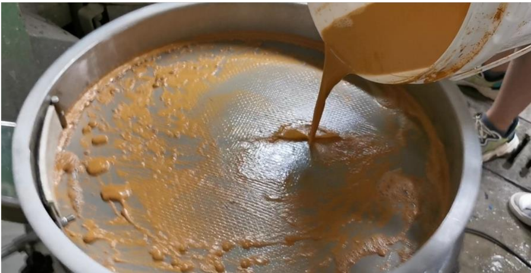
Plate 3: Step II for washing and sieving soil slurry into fine sand and mud slurry with water
