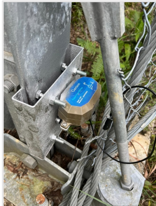
Plate 2: Photo of Sensor Fixing to Steel Post
