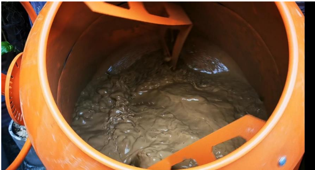
Plate 1: Step I for mixing and washing soil with water
