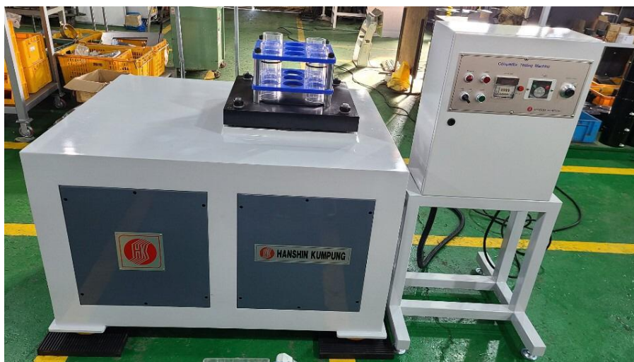
Figure 3: Compaction table for DCM laboratory mix test
