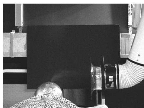
a Hood Position x = 0.3 \text{ m} , y = 0 \text{ m} ; Orientation \theta = 0^\circ
