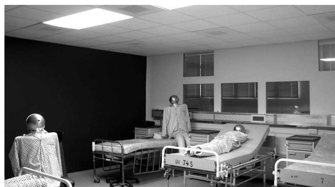
Figure 6 – Test Chamber and Manikins Modeling a Hospital Ward
