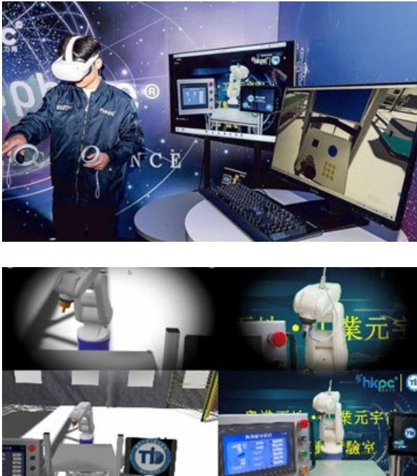
Figure 3. Remote Industrial Robot Teaching enabled by VR.
