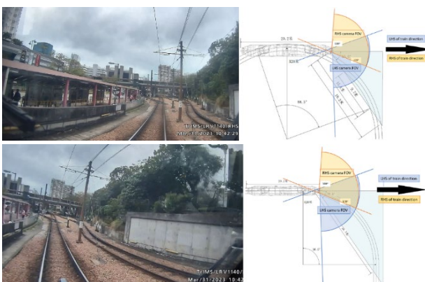
Figure 3. Dual camera Field of View (FOV) – Left and Right.
