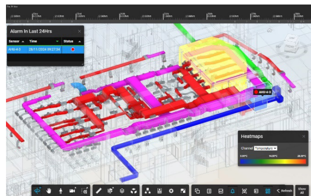
Figure 7. Integrating iBMS with the BIM-AM System to create a Digital Twin.
