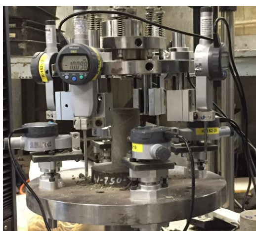
Figure 5. Compression test device.
