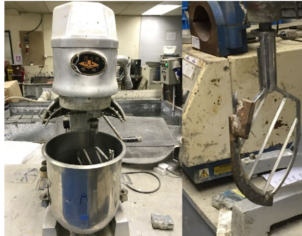
Figure 2. Mixer and paddle of flat type.
