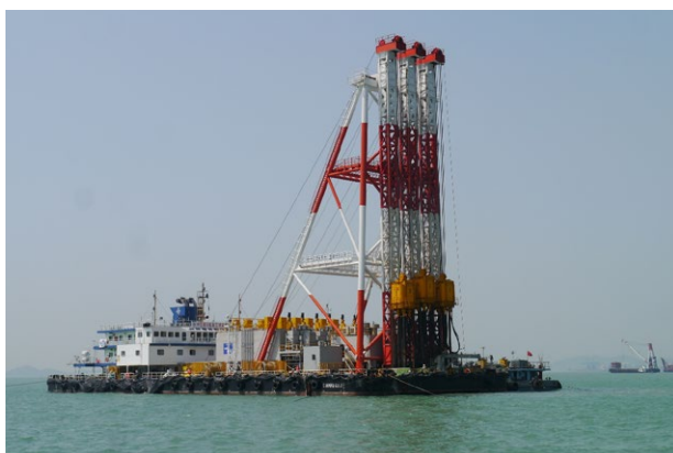
Figure 10. DCM barge operating offshore.
