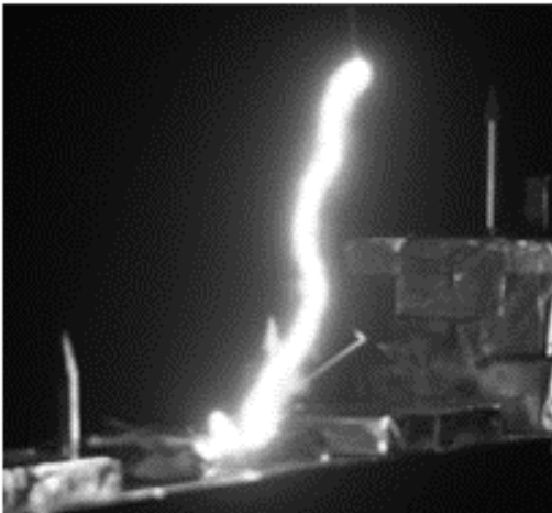
Figure 12. Discharge photo of the needle to the module.
