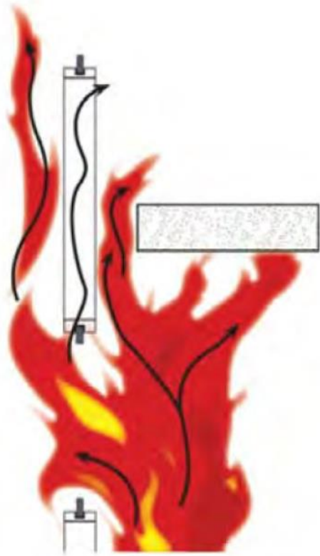
Unprotected Perimeter Joint
