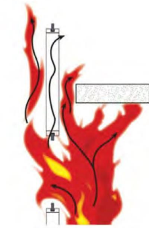
Unprotected Perimeter Joint
