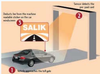
Figure 3.3.8 How “Salik” works [5]
